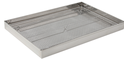
BABA DRAINING BOX Or candy rack. Consisting of a watertight stainless steel tray with a special grid with narrow mesh 9x9 mm (1/3" x 1/3"). Stainless steel frame with three 6 mm (1/4") cross pieces, 1 mm (3/64") wire, with feet.
